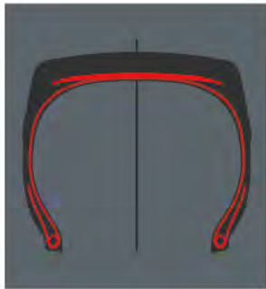
Tough casing construction for enhanced impact and cut resistance support
